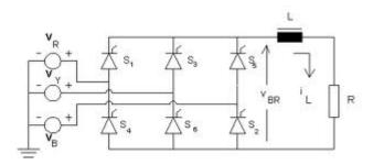
Figure 1. 3-phase fully controlled rectifier
